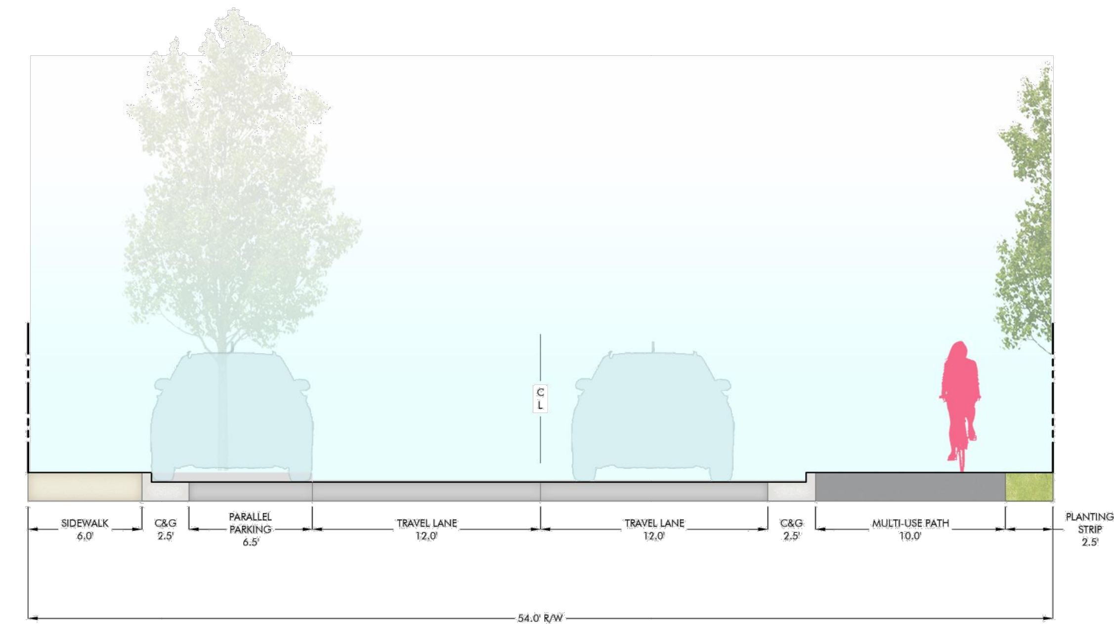
LOCAL STREET PARKING - GREENWAY CONNECTOR SECTION SCALE: 1" = 5'-0"
