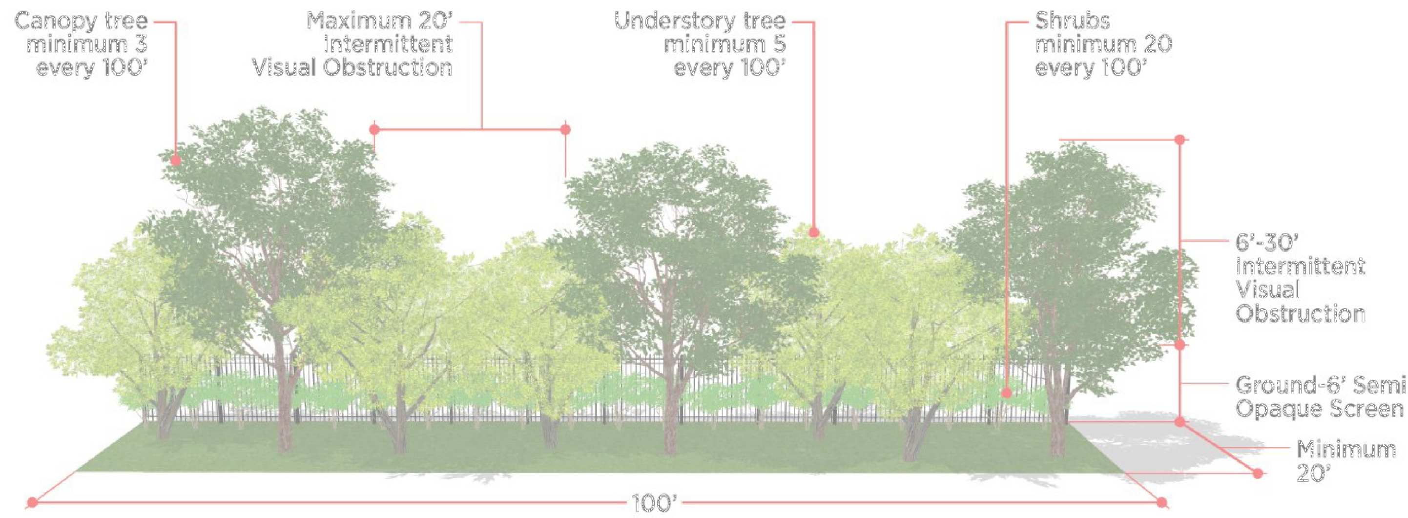
20' TYPE B PERIMETER BUFFER
